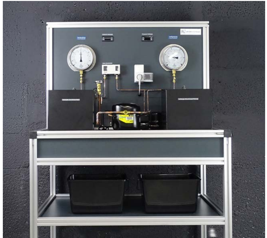
Training station Heat pump, water-water
