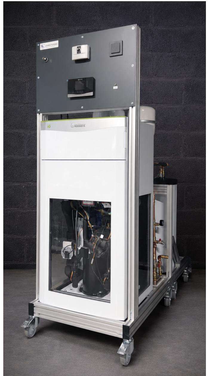
Training station Heat pump
