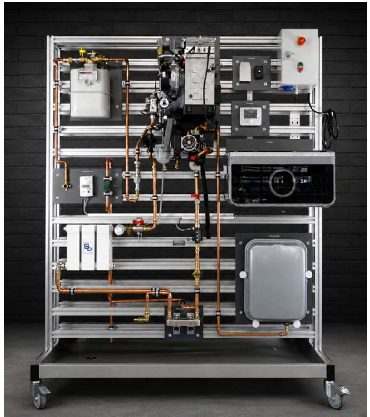
Training stand combined gas boiler
