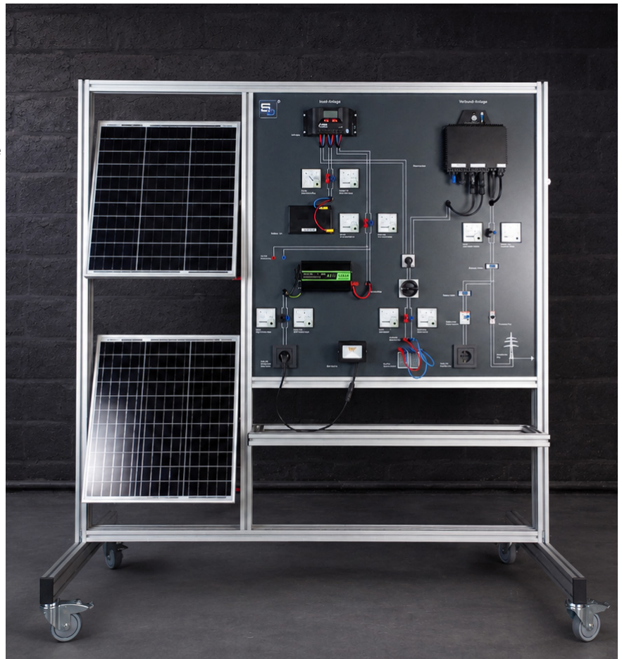
Training stand solar installation photovoltaic
