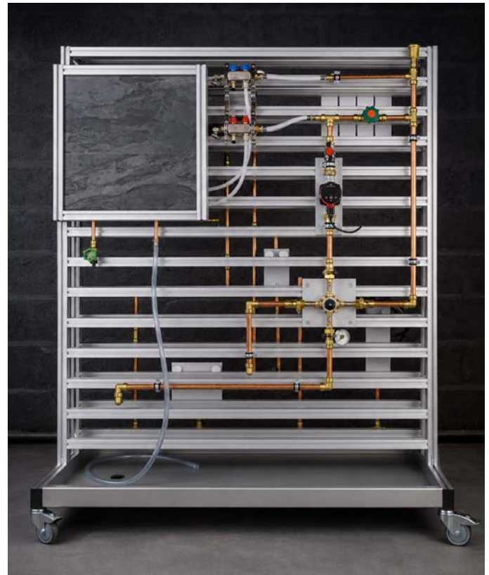
Module kit Heating extension mounted on trolley E-571730
