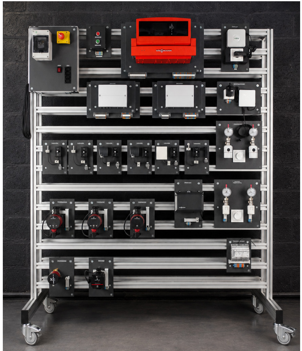
Heating Control Training Stand with original components, Viessmann controller, and extension kit for smart heating control, mounted on the Experiment and Assembly Trolley Art. No. 571730
