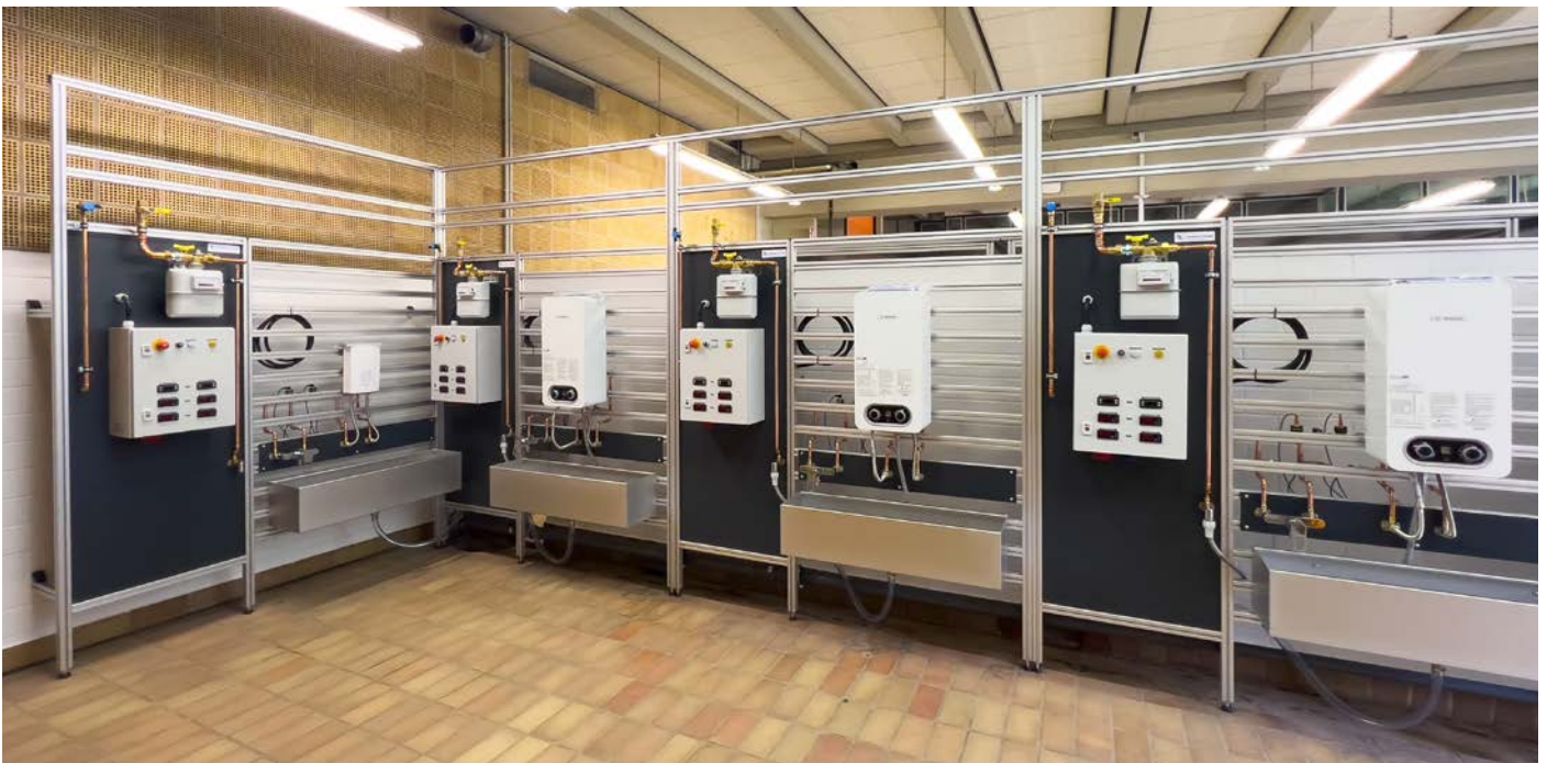
Example of a classroom installation: Test stands for gas and electric instantaneous water heaters
