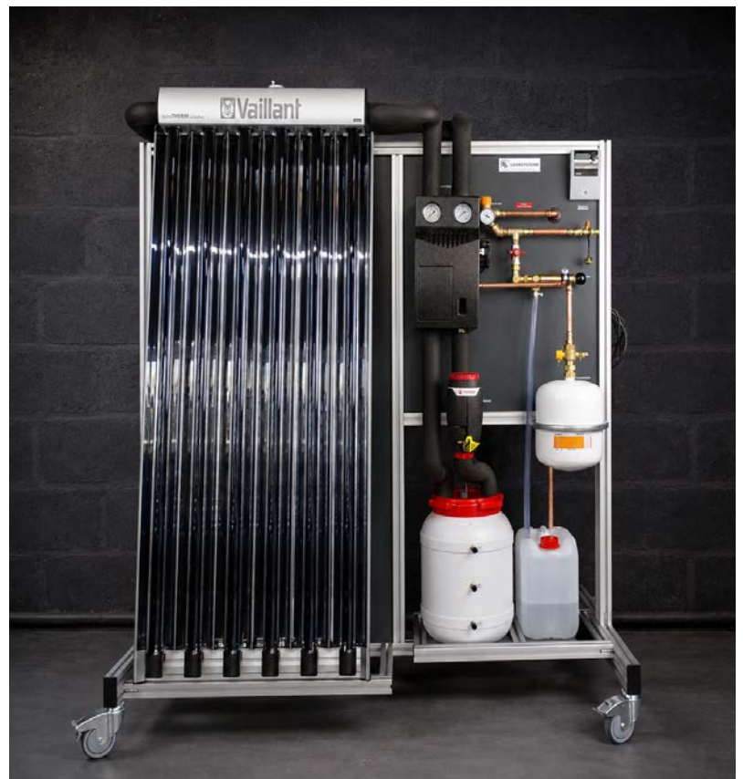
Training stand Solar system, tube collector
