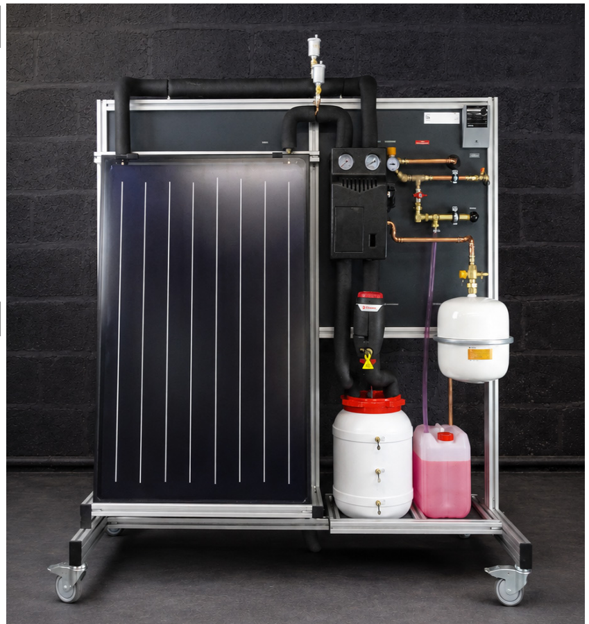
Training stand Solar system, flat plate collector
